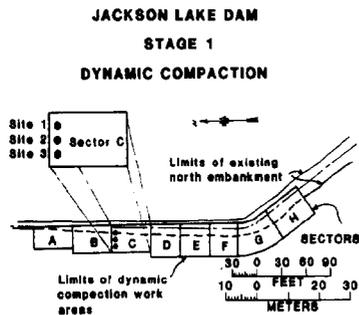
FIG. 1. Location map for crosshole test sites at Jackson Lake dams site, Wyoming.
