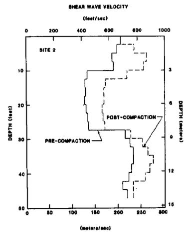
FIG. 3. Site 2 shear wave velocity profile.
