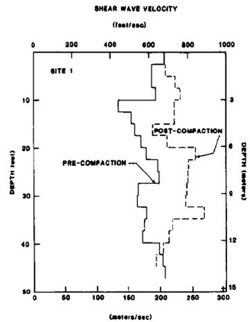
FIG. 2. Site 1 shear wave velocity profile.
