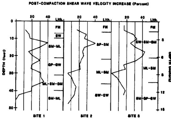
FIG. 5. Percent increase in shear wave velocities after dynamic compaction. Lithologies are presented in the Unified Soil Classification system.
