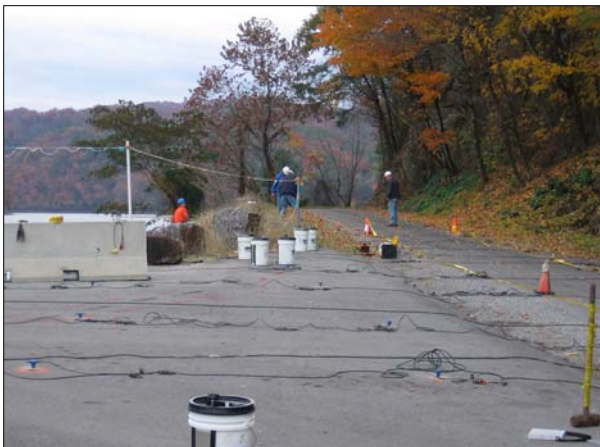
Photos: SP upstream embankment slope (left); SP off-shore (right); Seismic on crest road (bottom)
