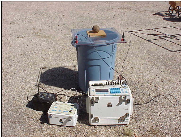
Figure 6: Photograph showing the major components of the fast TEM system used to acquire experimental data. The system is shown connected to a small (.5m x .5m) transmitter coil used for characterization measurements on small targets.
