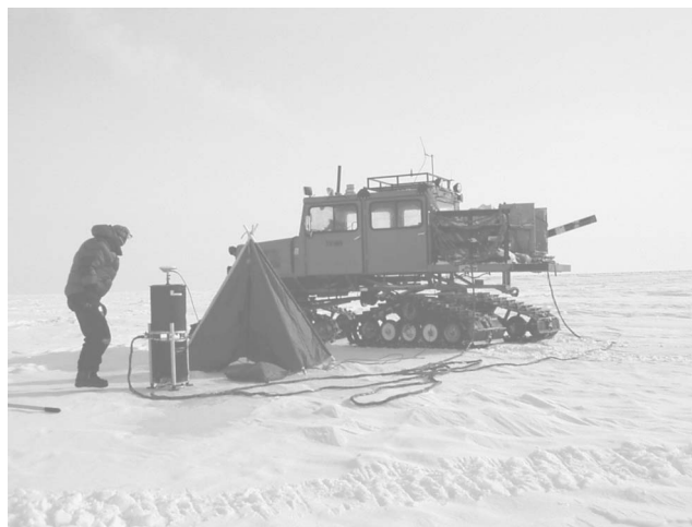
Figure 4. The absolute gravity meter deployed from a vehicle and ready to acquire data. The GPS antenna is mounted directly on top of the meter. The tent will be set up over the instrument to block the wind. Size and portability of the instrument are evident in the photograph.
