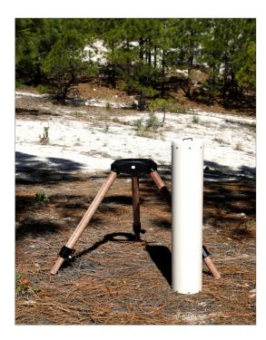
The TEM/3 antenna is a single channel, magneticfield antenna designed specifically for transient electromagnetic (TEM), controlled source audio-frequency magnetotelluric (CSAMT), and other types of EM geophysical surveys that require measuring vertical or horizontal fields.
