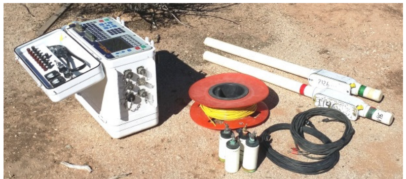
Zonge's backpack portable AMT acquisition system allows for use in difficult terrain and relatively easy field logistics.
