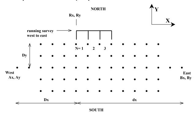
The AB transmitter dipole is set up on grid line 52,000 N, a-spacing = 50 m, the north-south baseline runs through the middle of the array, so that A is at -350 meters (350 W) and B is at +350 meters (350 E). The first potential electrode as shown is located at -100 meters (100 W), and 100 meters north of the transmitter dipole, or 52100. The data would be input as follows:
