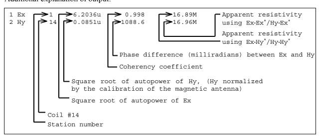
If you want to view the stored data, press the F7 key. It will display the last stack taken. See **Section** 7 for an explanation of the data mode. The data display is in the following format:
