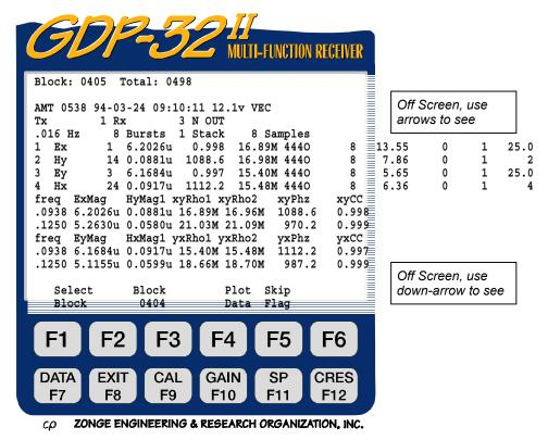
The BURSTS saved, SP, contact resistance values, pre-amp gain, variable A-spacing and reference channel have been saved, but are off of the screen to the right.
